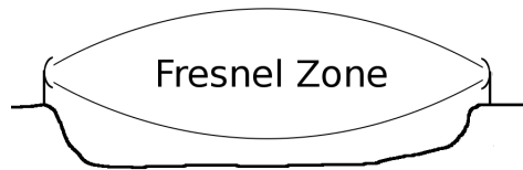
Figure 4: Fresnel Zone - Notice it is not just a straight line from one end to the other, it widens the farther you go from both ends.
